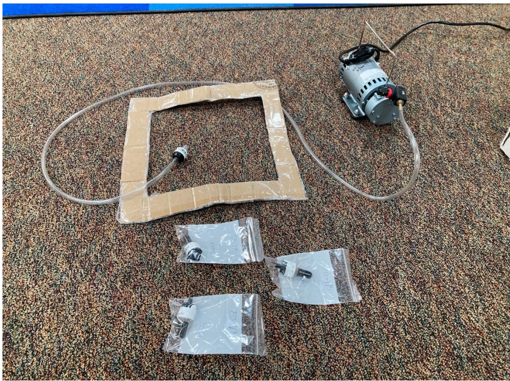
Photo 8: Microvac setup including cassette attached to a vacuum air pump, 1 square foot template and previously collected samples in bags.
