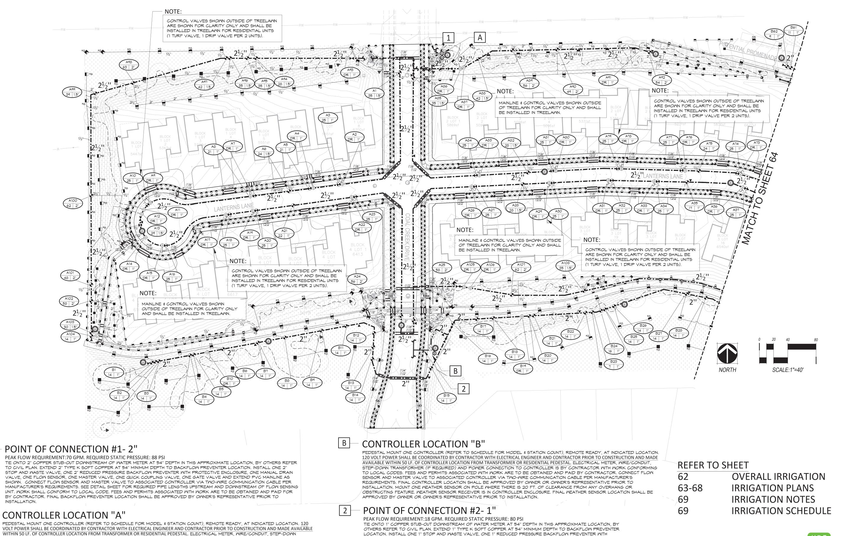
PROTECTIVE ENCLOSURE, ONE MANUAL DRAIN VALVE, ONE FLOW SENSOR, ONE MASTER VALVE, ONE QUICK COUPLING VALVE, ONE GATE VALVE AND EXTEND PVC MAINLINE AS SHOWN. CONNECT FLOW SENSOR AND MASTER VALVE TO
