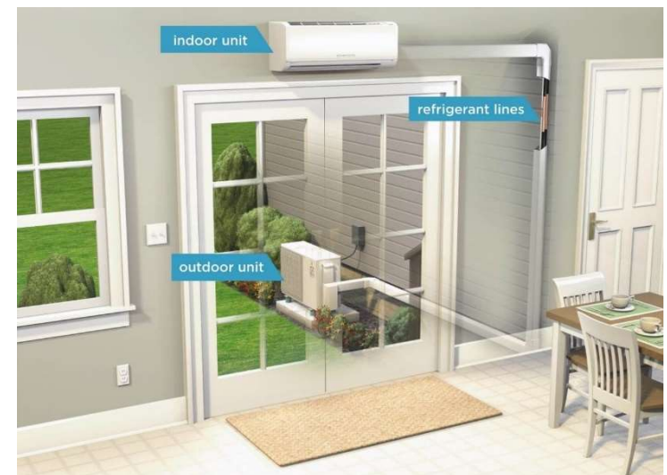
Mini-Split (ductless) Heat Pump (FAQs, wepowr.com )
