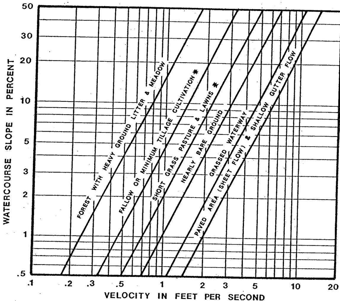
FIGURE 3-2. ESTIMATE OF AVERAGE FLOW VELOCITY FOR USE WITH THE RATIONAL FORMULA.
