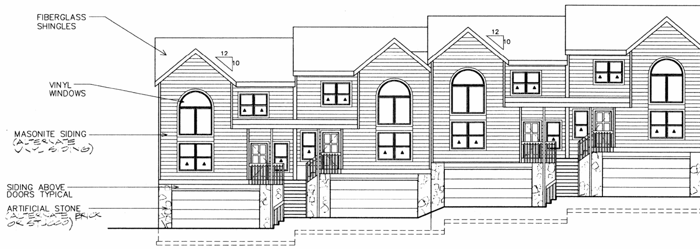
FRONT ELEVATION BUILDING 105
