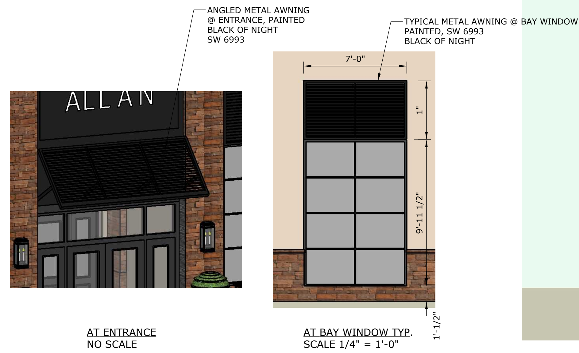
3 WINDOW AND AWNING SCALE: AS NOTED
