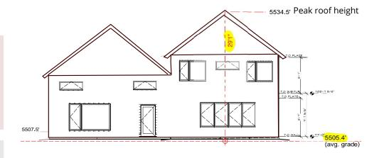
A plot plan is required to list elevation grades and reflect how average grade is calculated.
